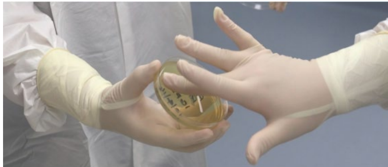
Figure 1. Gloved Fingertip Sampling Test Administration
